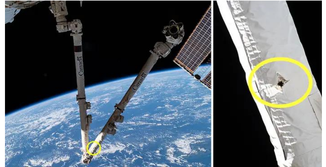
Damage to the ISS robotic arm by space debris ( businessinsider.com )
