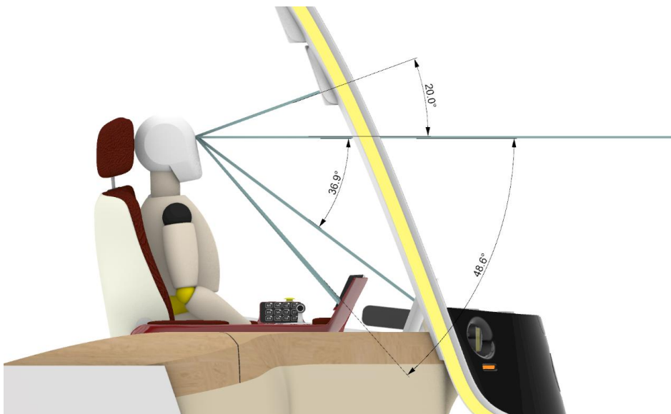
Fig. 6- 36 Side view of displays and controls
