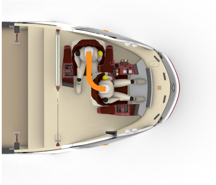
Fig. 6- 19 Driver seat movement
