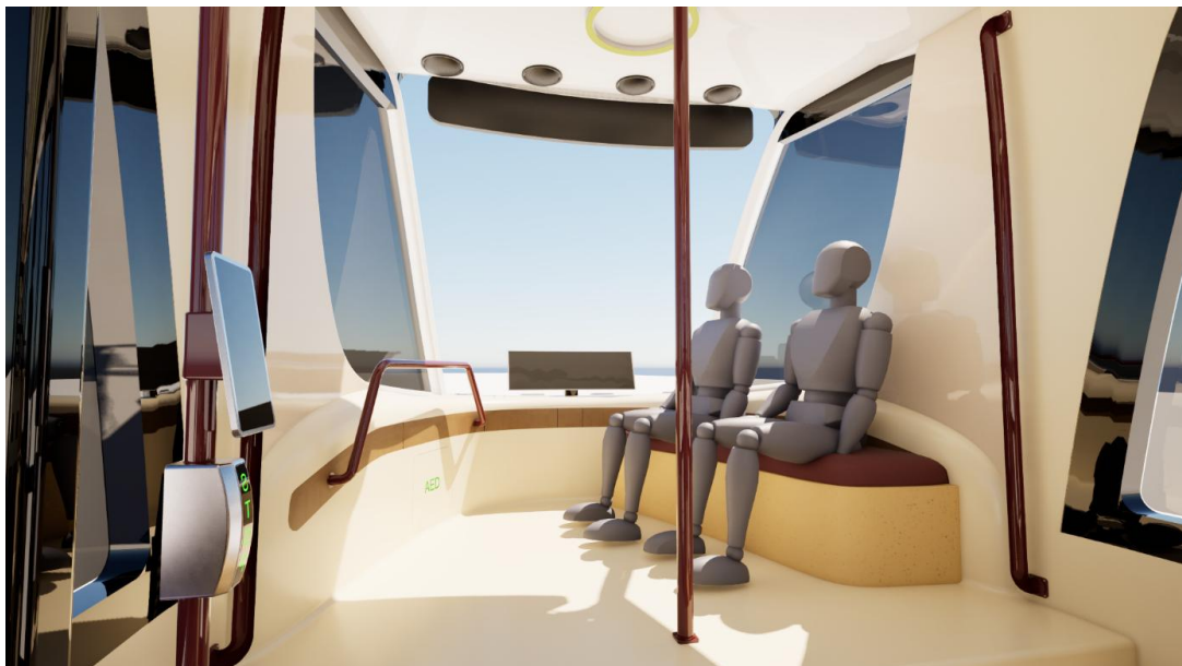
Fig. 6- 21 Modular cabin conversion from driver's cabin to passenger space
