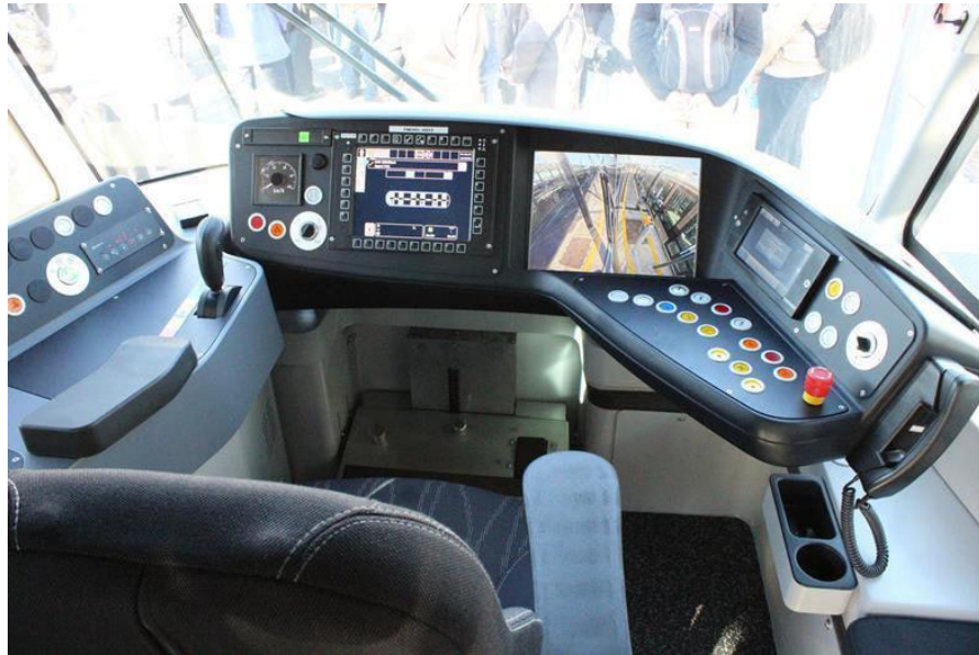
Fig. 2- 28 Driver's cabin of the Alstom Citadis TW20 Paris [29]
