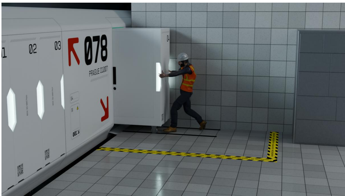
Fig. 6-16 Manual unloading operation at metro platform
