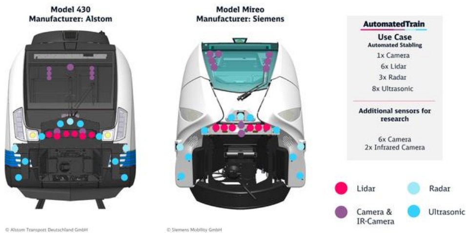
Fig. 2-36 Placement and types of sensors [34]
