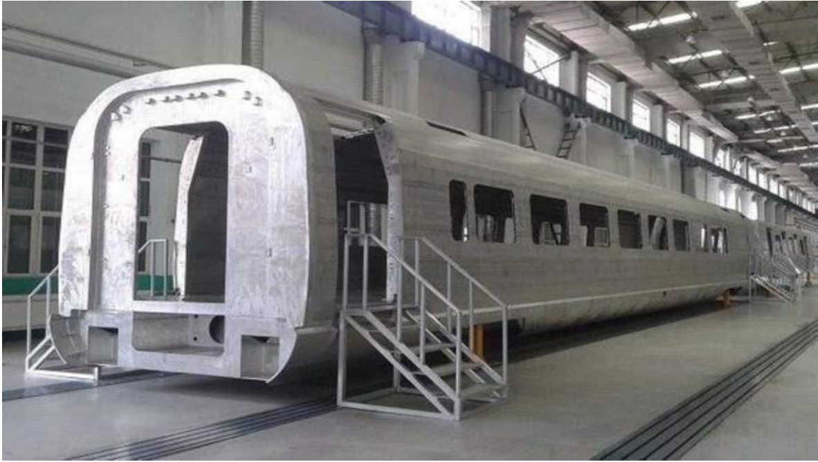
Fig. 2-32 Metro car body structure [33]
