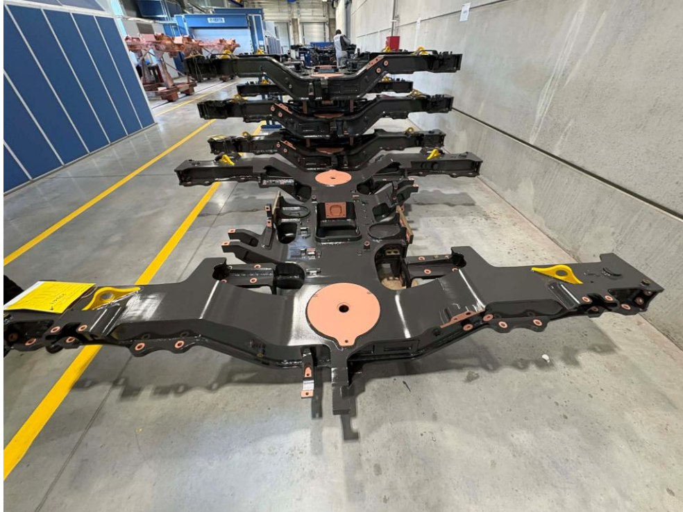
Fig. 2-30 Škoda Group metro bogie
