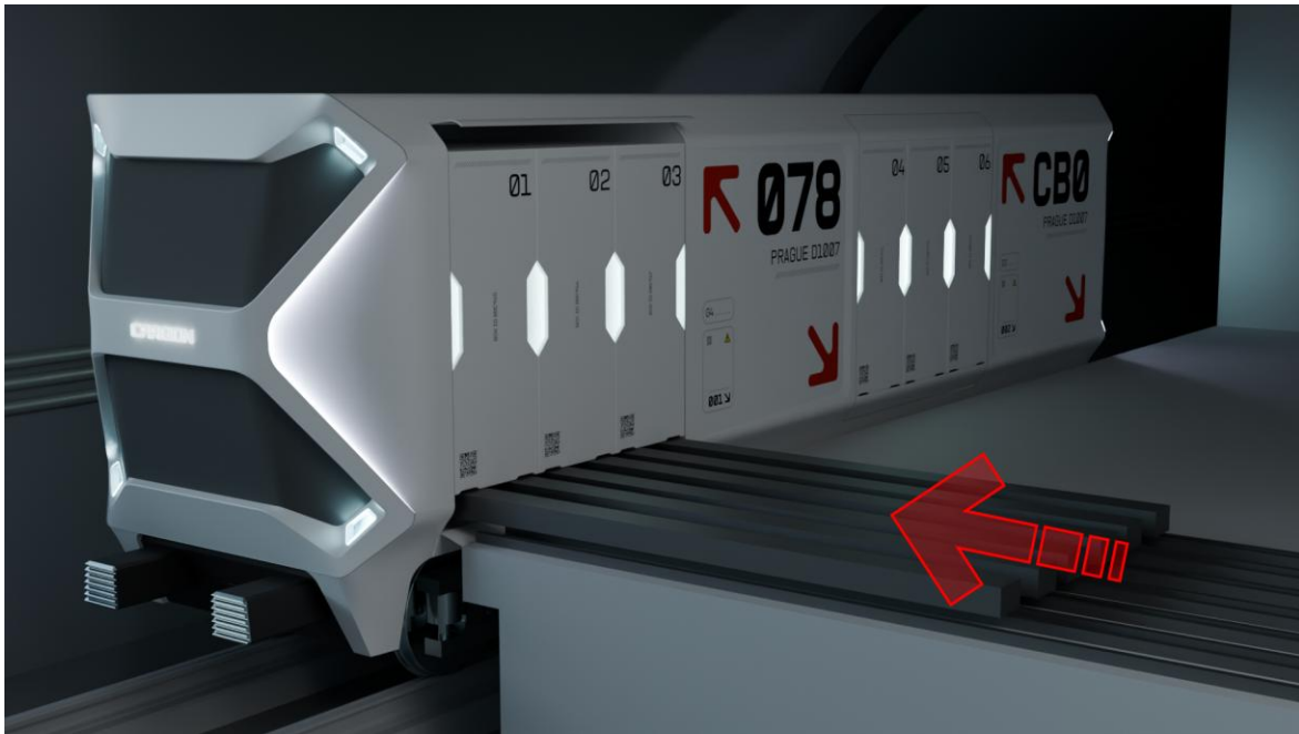
Fig. 6-6 Q-loader rails moving underneath the cargo boxes
