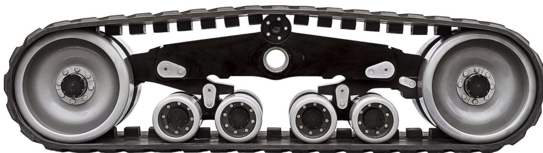
Obr. 2-17 double oscillating bogie suspension [29]
