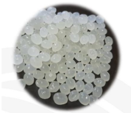
Obr. 4-2 Tvar granulátu Fillamentum PLA Natural [72]
