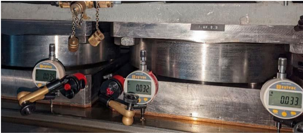
Figure 24 Setup for film thickness measurement by dial indicators [79].
