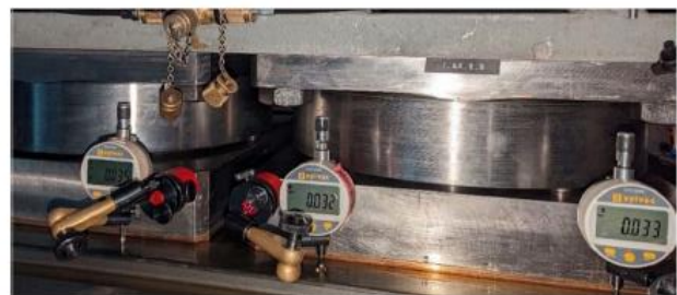
Fig. 5 Setup for film thickness measurement by dial indicators
