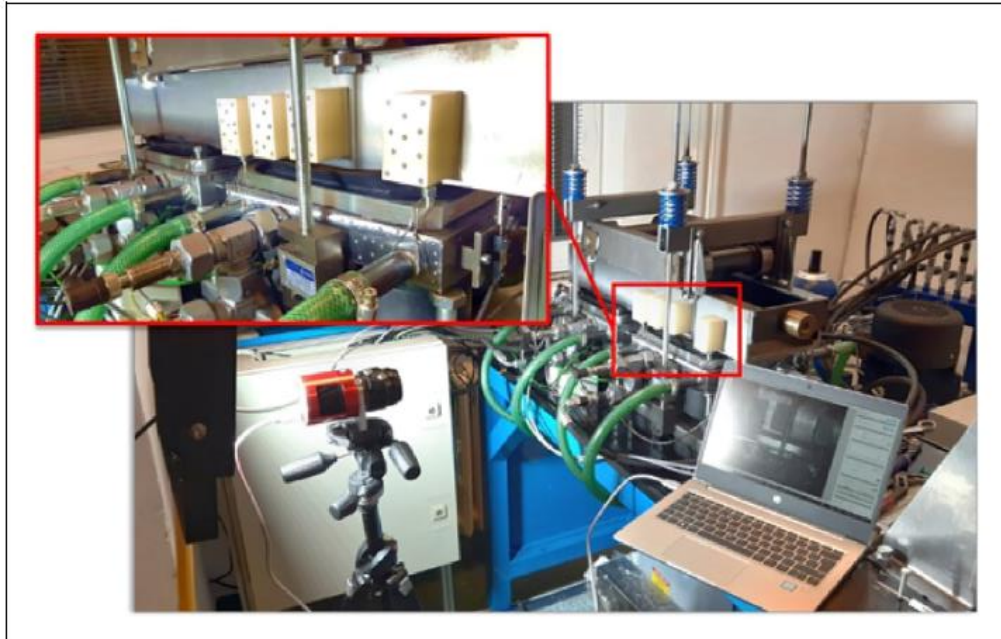
Figure 3. Experimental setup, detail of points on the bearing pad and slider, right – sample of measurement image.
