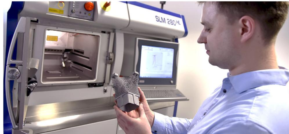
Additive Manufacturing of Metal Parts
