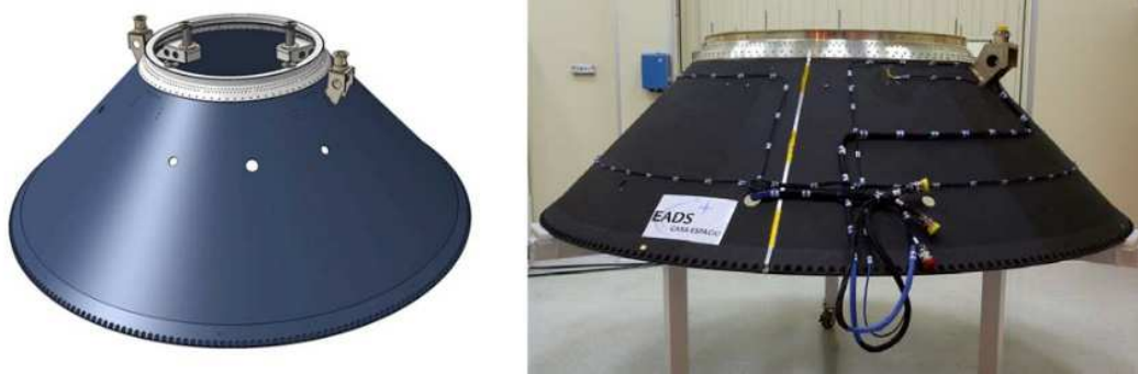
Fig. 10 ESA adapters: PAS 937C (left) [16] a PAS 1194C (right) [19]
