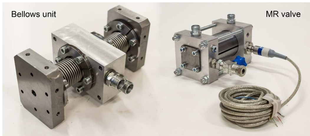
Fig. 66 Important parts of the experimental MR strut
