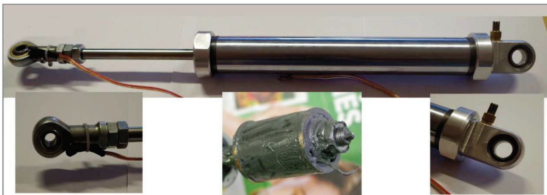
Figure 76 The design of MR damper
