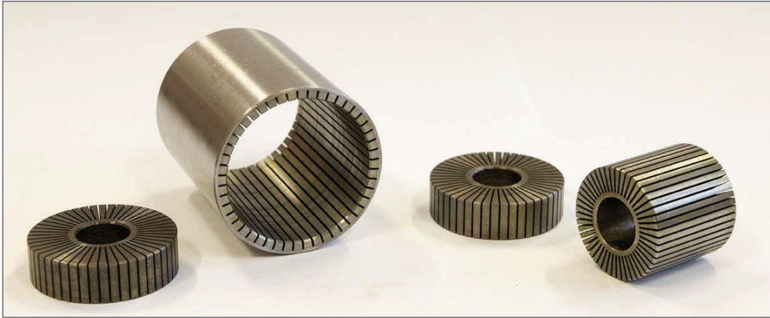
Figure 42 Manufactured grooves on the geometry of the MR damper
