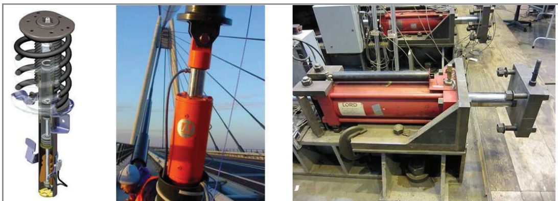
Figure 1 MR dampers (left) automotive [8], (middle) cable stay bridges [9], (right) damper for earthquake hazard mitigation [10]
